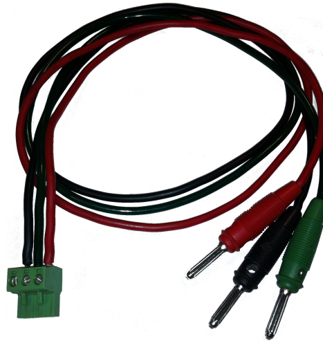
Figure 2: Three-wire power cable for the signal generator board.
